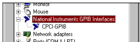
Figure 2-5. GPIB Interface That Is Working Properly
